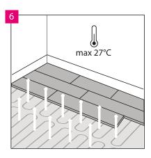
The floor panels may be applied on the substrate with underfloor heating, provided that the maximum temperature of the substrate surface is maintained at the level of 27°C. The underfloor heating must be switched off one day before the installation, and after the panels are laid, wait for another day and gradually switch on the underfloor heating [5°C per day].
