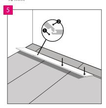
Then, snap the ribbon on to the previously laid rows with the long side.
