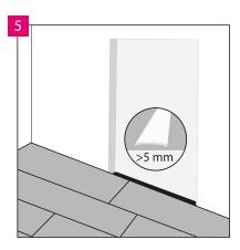
The application of the 5 mm expansion joint in the door opening between the rooms, which allows for the elimination of stresses, is recommended in the following cases: the irregular shape of the floor surface in the neighbouring rooms, the placement of heavy furniture in one of the rooms or the application of the underfloor heating only in one of the joined rooms. In the case of an area bigger than 200 m² or longer than 20 m, the expansion joint must be enlarged to 10 mm.
