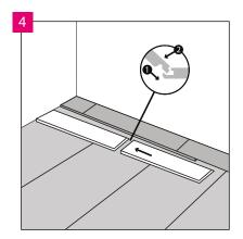
The floor panels are provided with locks on the short and long side. First, join the short sides of the neighbouring panels together.
