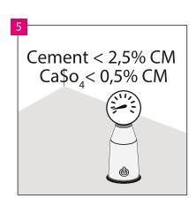
In the case of the cement grout, the moisture content in the substrate must be lower than 2.5%, and in the case of the anhydrite grout, it must be lower than 1.5%. In the case of installation with the underfloor heating, the above-mentioned values must be 1.5% and 0.3% respectively.
