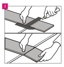
For additional cutting of floor panels, use a sharp knife, cut the top layer, then break the panel by leaning it on the edge. The floor panels may also be easily cut using an electric saw.
