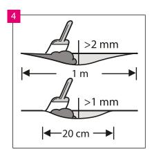
Make sure that the substrate is completely flat. All substrate irregularities exceeding 1 mm, with a length greater than 20 cm, or exceeding 2 mm with a length greater than 1 m must be levelled. Check if the use of the priming or sealing material is necessary. In order to prepare the substrate perfectly, spread the grout or the self-levelling compound on the
