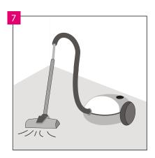
Make sure that the substrate is dry, flat, stable and free of any grease or chemical substances. The protruding irregularities must be scratched off and removed.
