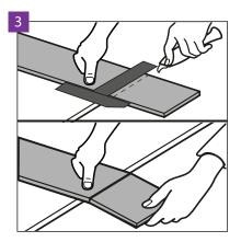
For additional cutting of floor panels, use a sharp knife, cut the top layer, then break the panel dynamically by leaning it on the edge. The floor panels may also be easily cut using an electric saw.
