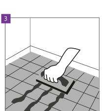
In the case of installation on the substrate covered with ceramic tiles, fill the tile joints with the gap wider than 4 mm and deeper than 1 mm with a durable compound for the filling of points, e.g. resin grout. Installation is allowed on tiles with grouts not wider than 5 mm and 1 mm deep without using levelling compound, provided the Multiprotec Hardlay or Vinclic Solid are used as underlay.
